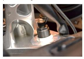
This photo shows the lower part of the rear shock. The rebound adjuster is the screw facing the camera toward the bottom of the shock. The preload adjuster is a large knurled knob not shown in this photo.
